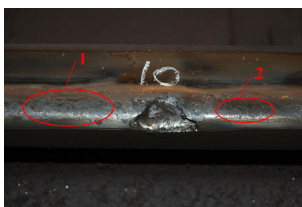
Fig. 3. The process of the crumbling depth development by code 11 based on the calculation.
